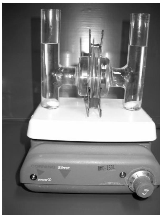
Figure 1 The modified dialysis apparatus used to prepare the A/C membrane.
